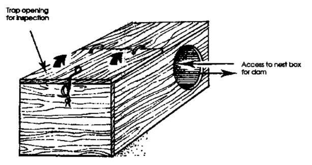
Note: In hot climates the top of the box can be made of wire mesh.
