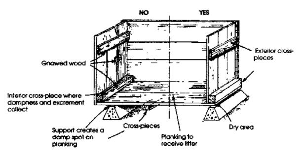
FIGURE 26 Examples of correct and incorrect cage assembly, fostering good hygiene and resistance (b)
