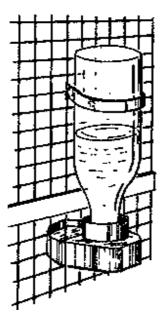
Automatic drinkers are fed by water from a low-pressure tank 50 to 150 cm above cage level. This tank can be used to administer medicine with the water. It is usually filled either by water under pressure (automatic watering) or manually (semi-automatic watering). The tank must be in the shade so that the water will not heat, which would be bad for the rabbits. Further solutions are seen in Figure 31.
